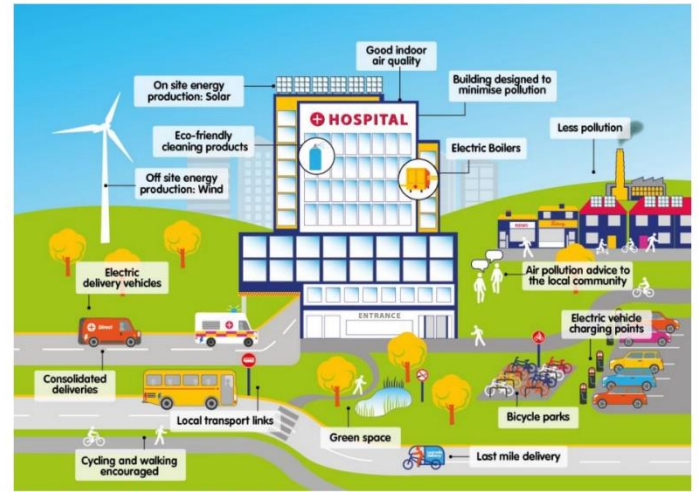
Figure 2: Example features of a clean air hospital
