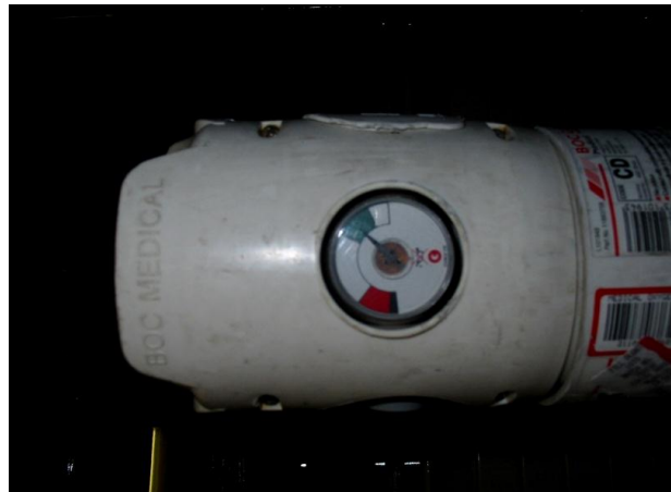
A CD cylinder on side displaying contents gauge . The contents gauge needle indicates that the cylinder is full (green).
