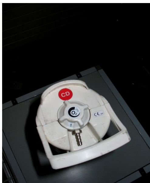
The flow valve is turned on to 1 litre per minute
