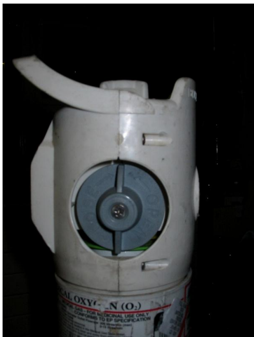
The CD Oxygen cylinder valve is closed The valve is turned clockwise
